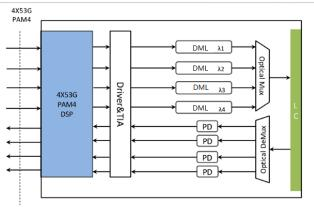
Figure 1. Transceiver Block Diagram
