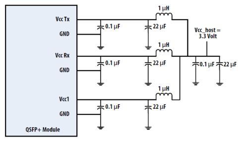
Figure 3. Recommended Power Supply Filter
